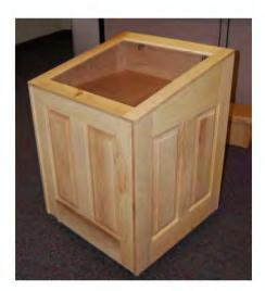
The Illinois Department of Agriculture and the University of Illinois Extension in cooperation with the Illinois Department of Transportation have commissioned the building of 33 kiosks made with reclaimed ash wood. The wood, taken from an EAB-infested IDOT Rest Stop along I-57 in Loda Illinois, was harvested, milled and made into lumber for the project.
